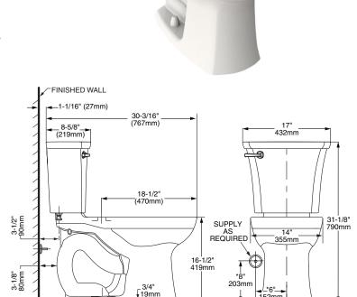
THIS TOILET IS DESIGNED TO ROUGH-IN AT A MINIMUM DIMENSION OF 305MM (12") FROM FINISHED WALL TO C/L OF OUTLET. SUPPLY NOT INCLUDED WITH FIXTURE AND MUST BE ORDERED SEPARATELY. \* DIMENSION SHOWN FOR LOCATION OF SUPPLY IS SUGGESTED.
