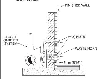
Using a level, adjust the top left back-up nut so that it is in the same vertical plane as the lower left back-up nut.
