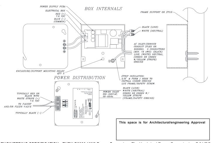
**ENGINEERING SPECIFICATION: ZURN P6000-HW6 Power Converter -** The Hardwired Power Converter is a 7.6 VDC regulated, 2.0A power supply that will operate up to: (8) ZEMS or ZEMS-IS Sensors/Actuators, (8) ZESS Sensors/Solenoids, (8) sensor faucets, or (8) Pint Urinal valves. The unit shown above is integrated into a 4"L x 4"W x 2-1/8"D electrical box. The AC input connections are terminated within the electrical box. The 7.6 VDC output terminals are externally mounted to the cover plate.
