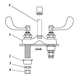
3. Place no.1 into holes in sink top and replace no.2, no.3 and no.4 onto threaded shank. Tighten no.4 firmly with a wrench.
