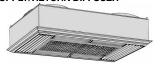
Designed to convert a side by side or an over and under arrangement into a concentric distribution of air. The diffuser is flush mounted, completely insulated, assembled, and internally baffled to provide four way supply air distribution with a center return. To make the assembly complete and ready to fit into a 2' [0.61 m] x 4' [1.22 m] suspended ceiling grid, the diffuser includes adjustable supply louvers, hanging rings, anti-sweat gasket, and round flanges for use with flexible ducts.
