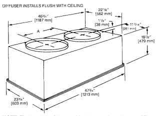
**NOTE:** The location of the combination supply and return diffuser should not exceed 10 feet [3.05 m] above the floor level for units @ 1000 CFM [472 L/s] or less and 12 [3.66 m] to 14 feet [4.27 m] above the floor level for units with CFM greater than 1000 [472 L/s]. If the diffuser is installed with a greater distance than recommended above, the supply air may become stratified above the required comfort area causing uncomfortable conditions.
