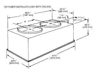
**NOTE:** The location of the combination supply and return diffuser should not exceed 10 feet [3.05 m] above the floor level for units @ 1000 CFM [472 L/s] or less and 12 [3.66 m] to 14 feet [4.27 m] above the floor level for units with CFM greater than 1000 [472 L/s]. If the diffuser is installed with a greater distance than recommended above, the supply air may become stratified above the required comfort area causing uncomfortable conditions.
