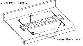
After making cuts along sides of cutout, secure a board as shown to prevent cutout from possibly damaging countertop or prematurely dropping.
