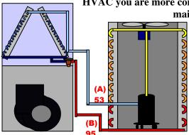
maintaining full capacity of the evaporator coil. Connecting a clamp thermometer in the shade, on the vapor line, will achieve this reading. Allow 5-10 minutes of run time to allow system to balance. For our example the Vapor Line
