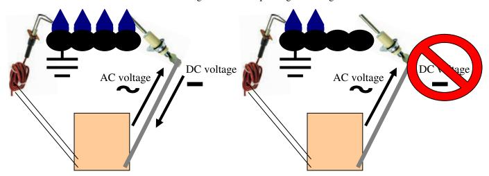
If the flame does not fully light the A/C current is never rectified and the circuit board does not see the burner ground.
