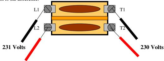
The proper way to check is to measure *across the contacts* <u>as well</u>. Any voltage reading of 1 or more volts indicates the contacts are not properly closing and should be <u>recommended to be replaced</u>. This 1 volt drop tells the technician that the switch has become a load and will produce heat. This will continue to heat up dropping more voltage until either it burns up the contacts or robs enough voltage from the compressor to possibly cause damage to it as well.
