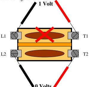
No measureable voltage should be read across the energized terminals of a switch or fuse unless it is open.
